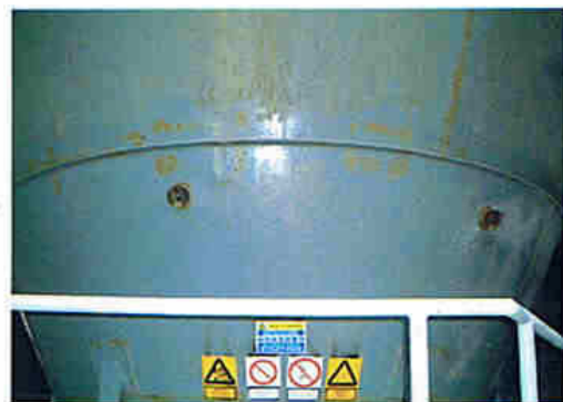
Above: Small Cardox Sockets are welded onto the cyclone and below the feed pipes.
