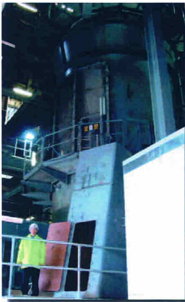
Above: Cardox Sockets in evidence on cyclone. Below: Danny Coulston by the 37.5 raw meal VRM. Which uses an 1835kW drive from ABB, running at 993rpm, and a MAAG gear, Bottom Right: The main 33kV to 11kV transformer on the site, supplied by On Load Gears, Chennai and Marson's Ltd, Kolkata.
