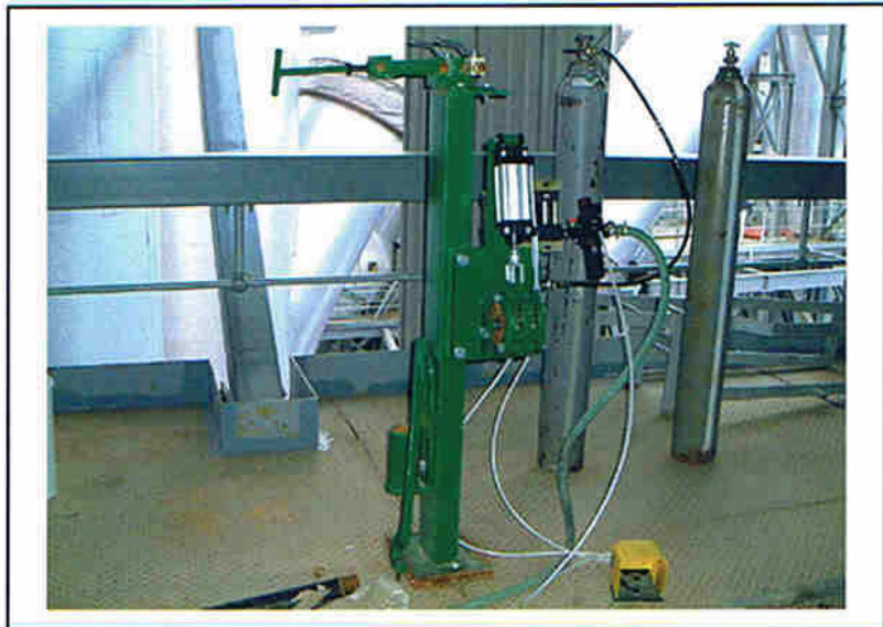
Above: The Cardox Recharging Unit can be located anywhere on the pre-heater and can even be portable.
