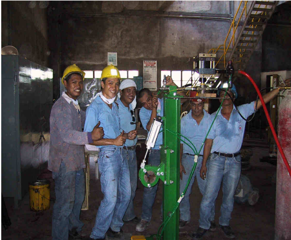
Plant Engineers give the 'thumbs up' for the Cardox System. The versatile System is easily installed and provides the most efficient, reliable and cost effective method of clearing build-ups and blockages. Photo depicts the compact Cardox Tube Recharging Unit.
