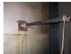
CARDOX tube is inserted in the tube holder and secured in the socket. Tube is then activated.
